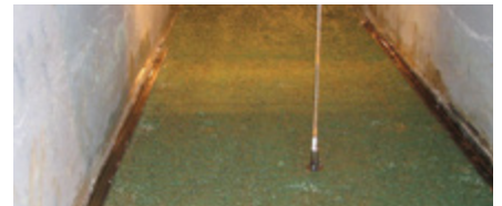
Post-test endurance results concluded that unvegetated GreenArmor 7020 exhibited a critical shear stress of 5.8 lb/ft 2 (280 N/m 2 ).
