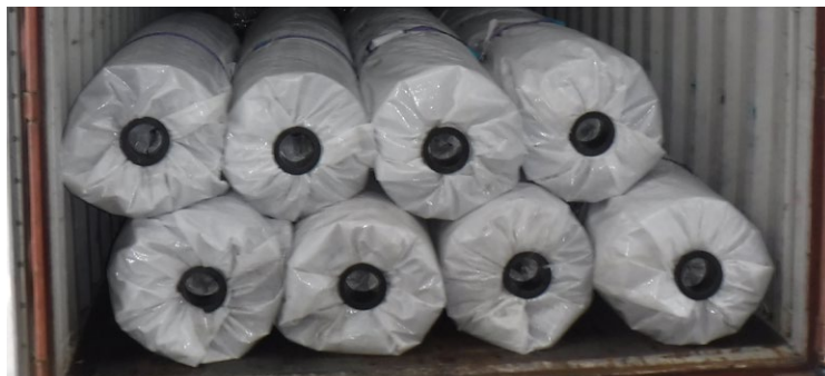
3-Wide 'end on' container loading
